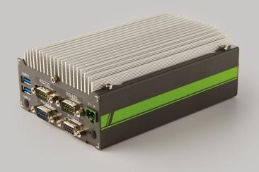
The VB-30 from Vemotion is a multi-channel hybrid recording and transmission unit supporting options for Analogue and IP, HDMI, HD-SDI inputs. It offers outstanding value and flexibility in a very small package.
